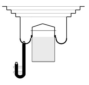
The second piece of the system is the media canister. It is made of corrosion resistant. PVC and is inserted into the center of the skirt. A gasket seal prevents air from bypassing the canister. The odorous air enters through the canister bottom, travels up through the media and is exhausted through the top cover.
